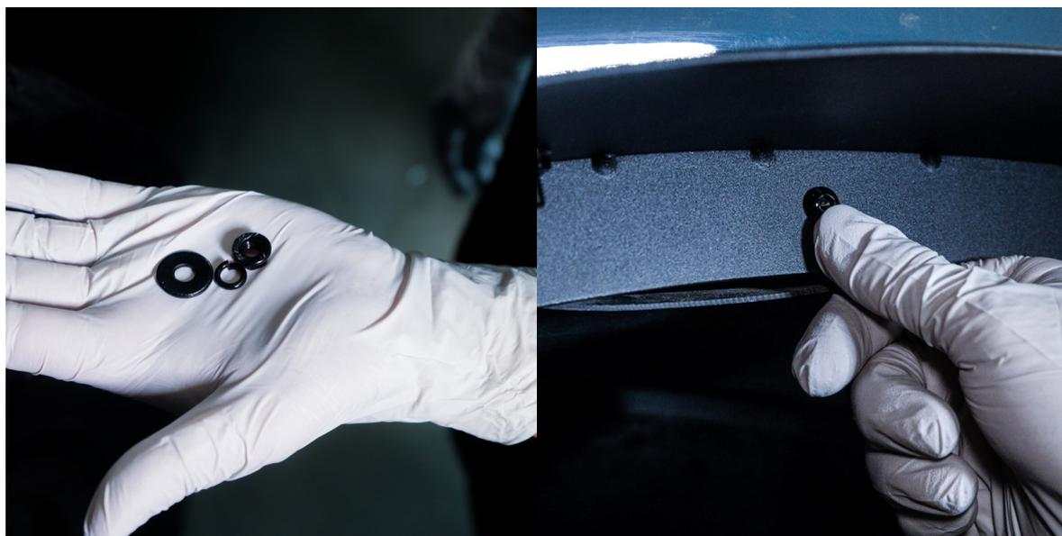
Attach the mounting points using **W09** and **W13** washers, **N09** nuts, and **B66** bolts. Secure them in place by tightening with a **10mm wrench** and a **4mm hex socket tool**.
