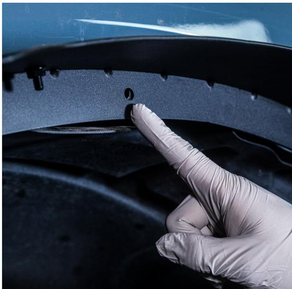
Align the fender flare with your vehicle's body, as shown on the left.
